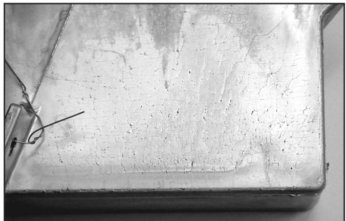
Figure 2-12 Washout as seen on a casting.
