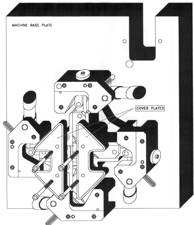
Figure 4B-7 Miniature die casting die shown with clamps.
