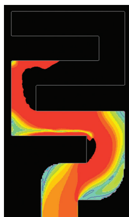
Figure 7-5a: Square corners in a runner or casting result in porosity pockets.
