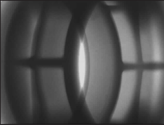
Figure 7-21A: Example radiograph of a casting with no visible porosity revealed by radiography. This level of soundness is achievable through consultation with your die caster and good part design, process design and process monitoring.
