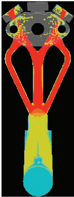
Figure 7-1: This is an example of the overflows filling first instead of being the last place to fill. An initial fast simulation will detect such undesirable characteristics.
