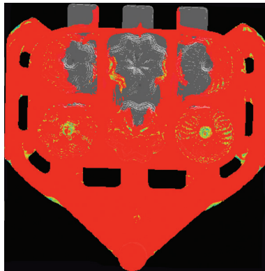
Figure 7-2: This simulation shows the end and top overflows are of no value. The cavity areas encircled are filled with porosity. The scrap rate was 75%. A new gate/runner with confirming simulations yielded a 1.5% scrap rate. The simulation will save hours of rework and lost time.
